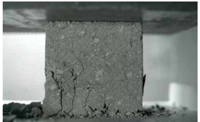
Cube crush - Strength test after 14 & 28 days
