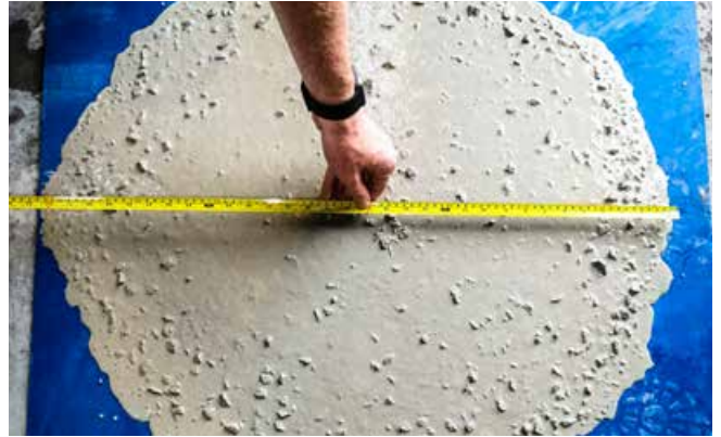
Flow test - Test moisture of self compacting concrete
