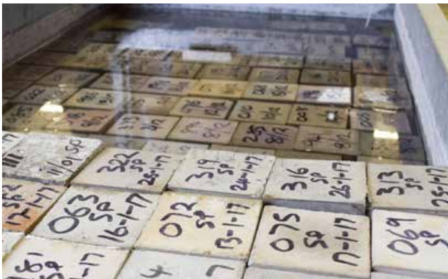
Concrete cubes - curing process before testing
