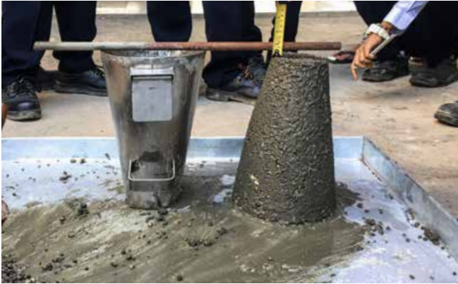
Slump test - Test moisture content of drycast concrete
