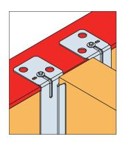
Fasteners to be installed through the inner obround slot in the hanger top flange.
