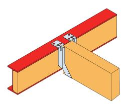
Timber in the flange of the 'I section steel beam is required when hanger depth is shallower than steel depth. Timber to finish flush with outer edges of 'I' section's flanges.
